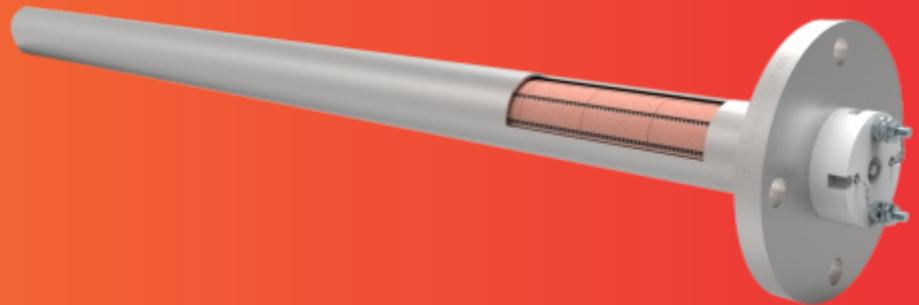
Bobbin heaters are mainly used for direct heating of air and indirect heating of liquids and gases where the element is fitted into a pocket in the process tank or system so that the element may be replaced without draining down the system or vessel. Highly energy efficient as heat is generated within the solution. Extensively used for transmission of heat, these heaters are available in various specifications that meet the individual necessity in the best possible manner.
